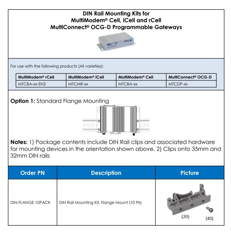
**Note:** An additional hole has been added to the mounting flange to support DIN rail mounting. MTCBA-xx products will begin shipping with the additional hold at the beginning of 2Q 2014.
