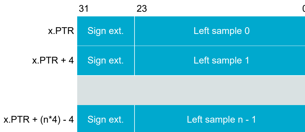
Figure 81: Memory mapping for 24-bit mono, left channel only. CONFIG.SWIDTH = 24Bit, CONFIG.CHANNELS = Left.
