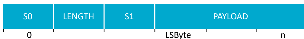
Figure 111: Representation of a RADIO packet in RAM
