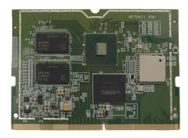
Introducing the AMPAK System on Module, featuring the Synaptics Astra™ SL1620 with Synaptics combo connectivity, which delivers exceptional capability and flexibility for applications such as medical data acquisition terminals, home control and automation, and home appliances
