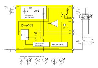
Figure 2: Integrated laser driver circuit
