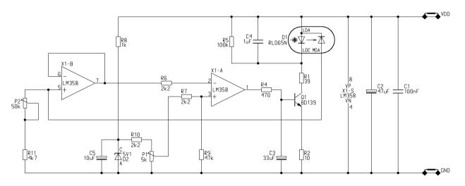
Figure 1: Typical discrete laser diode driver circuit\*
