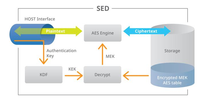
Unlike the software-based approach, the SED is encrypted or decrypted instantaneously, and there is no processing load on the main system CPU. When retrieved from the disk, data is decrypted locally and transferred unencrypted across the PCIe/SATA interface into the computer. The hardware-based approach's greater efficiency in mobile and portable equipment can help improve energy utilization and extend battery life.
