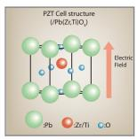
FRAM stores information using the polarization of ferroelectric material placed between two electrodes in the form of a thin film. The FRAM cell structure, which is similar to the transistor and capacitor structure of a DRAM cell, does not require the same high
