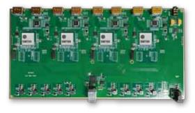
Fig.3: a reference design developed by Silicon Motion for an eight-display video wall box
