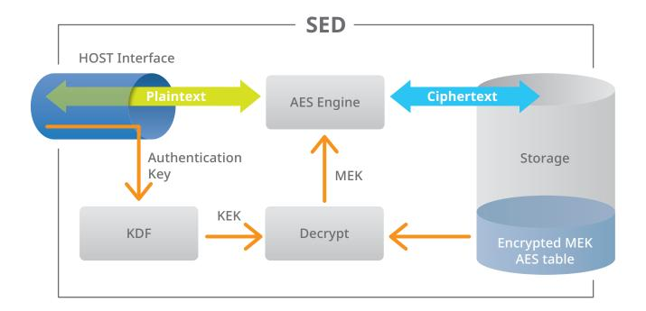
Unlike the software-based approach, the SED is encrypted or decrypted instantaneously, and there is no processing load on the main system CPU. When retrieved from the disk, data is decrypted locally and transferred unencrypted across the PCIe/SATA interface into the computer. The hardware-based approach's greater efficiency in mobile and portable equipment can help improve energy utilization and extend battery life.
