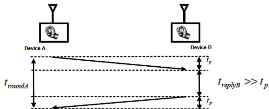
Figure D1.5—Exchange of message in two-way ranging
