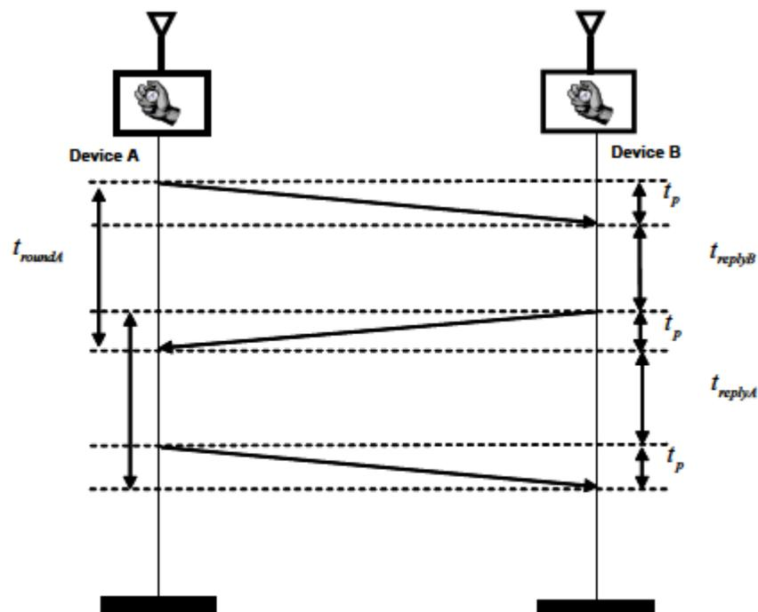
Figure D1.6—Exchange of message in SDS-TWR
