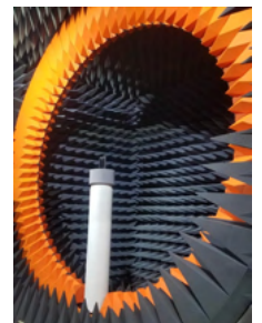
Anechoic Chamber 400 MHz - 18 GHz
