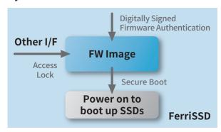
FerriSSD maintains boot security via secured digital signature authentication
