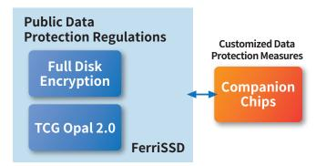
Full disk encryption is available via TCG OPAL. For optional added security, optional companion chips are added to enhance the security of sensitive user data.
