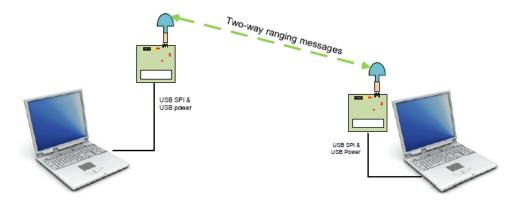
c. Using the external application to control one of the pair of the EVB1000 units.
