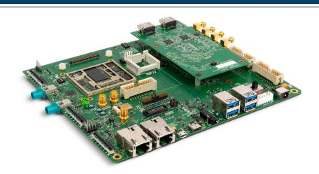
The Open-Q™ 8550CS Development Kit is designed to facilitate easy evaluation of the key features of the Qualcomm® Dragonwing™ QCS8550, such as the Low Power AI subsystem with a dedicated DSP and AI accelerator supporting always-on audio, sensors, contextual data streams, and an always-on camera. The kit supports the evaluation of C-PHY and D-PHY MIPI CSI and GMSL cameras, dual MIPI DSI, DisplayPort, audio, sensors, GNSS, Gigabit Ethernet and many more features.
