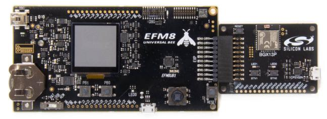
Figure 3.1. BGX Expansion Board Connected to EFM8
