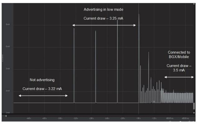
Figure 4.4. Energy Profiler Capture of BGX with 115200 bps UART Baud Rate
