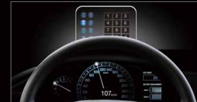
<A display cluster with an eco-drive assist function>
